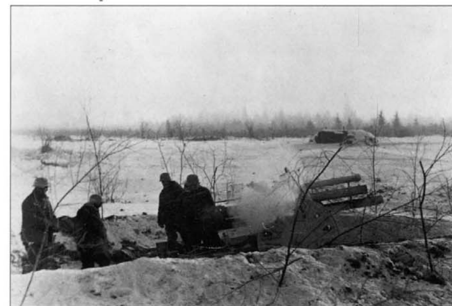
RIGHT: German artillery in action in January 1943. The gun is a 105mm leFH18 standard field howitzer, which was equivalent to the British 25-pounder. It was a versatile weapon, capable of firing all types of projectile and even knocking out tanks at short ranges.
