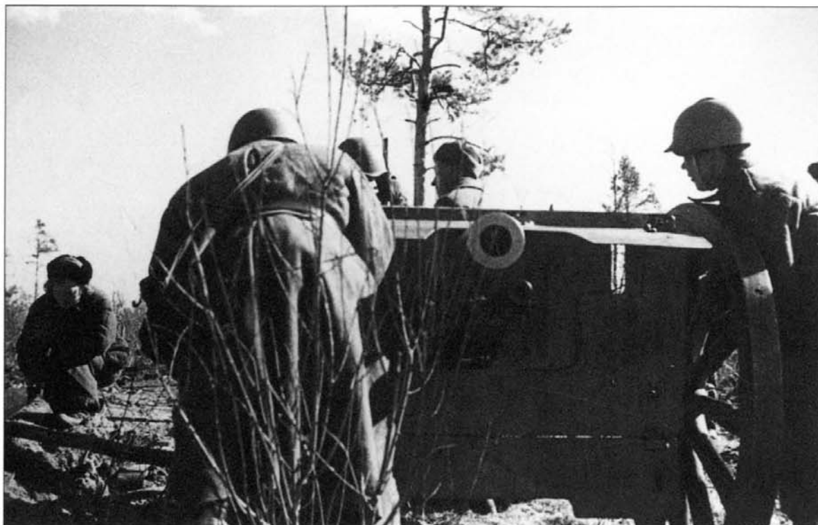
ABOVE: This artillery crew manhandles its 76.2mm field gun into a newly finished position. Although this model 1902 weapon was obsolete by 1941, many were pressed into service during the early months of the siege. The upper part of the shield has been lowered for ease of placement.
