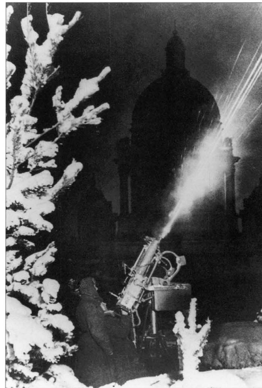
RIGHT: A beautifully composed image, more son et lumière than war. Silhouetted against the night sky is the dome of St. Isaac's cathedral in Leningrad. The weapon is the 4M, a special mounting of 7.62mm Maxim machine guns, which was the most common air defence piece in the Leningrad area.
