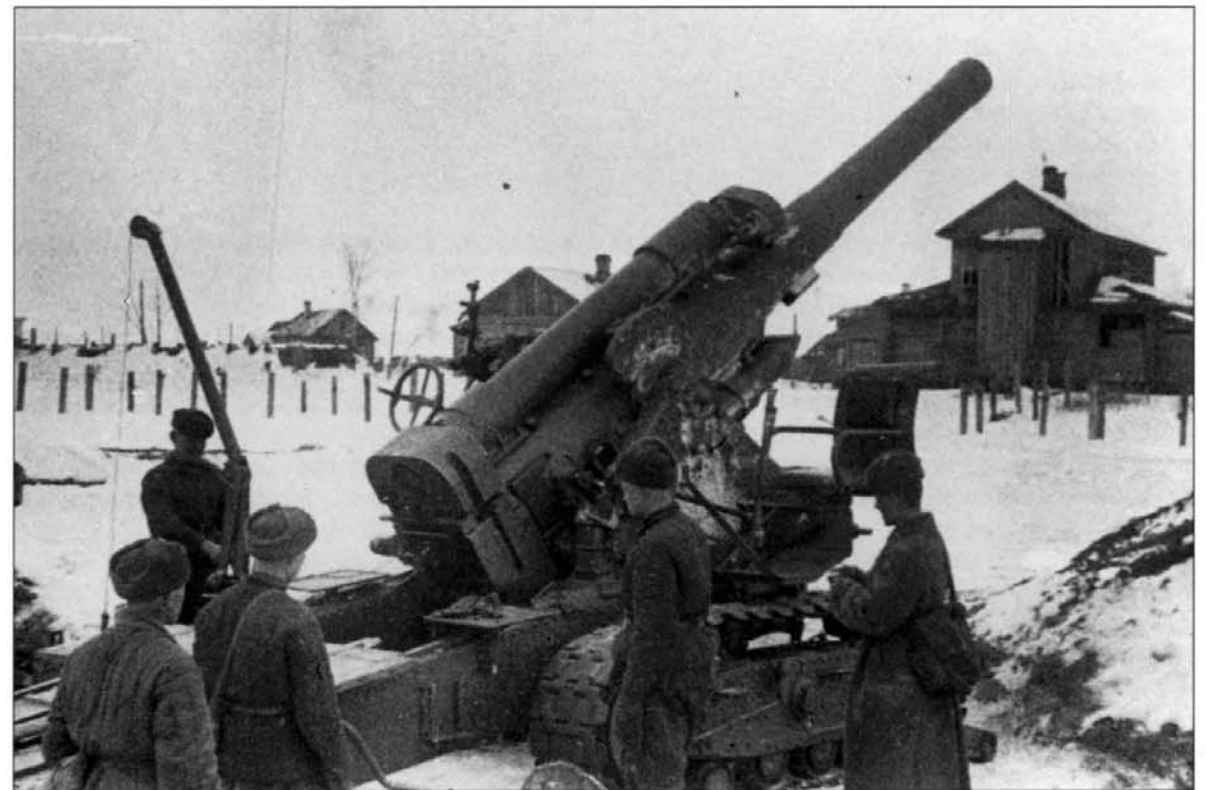
BELOW: As a counter to the siege artillery deployed by the Wehrmacht, the Red Army employed units of heavy artillery such as this 203mm howitzer, which has just been towed into place. To the left of the picture is the crane for lifting the round.
